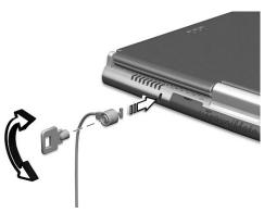
Wrap a computer security lock cable around an immovable object such as a table or locked drawer handle. Insert the lock into the notch and turn the key to secure the lock. Some keyless models are also available.
